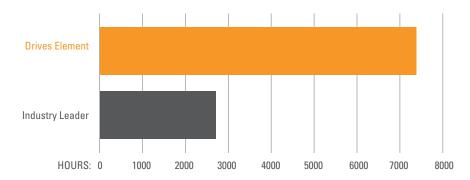
Accelerated wear test conditions: ANSI 60 chain, 275 RPMs, 230 lbs. (1023N) tension, 3.0 chain horsepower (2.24 kW), 23T x 23T sprockets.
