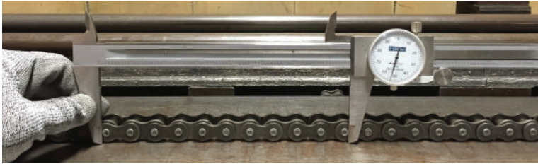
Figure 1: Measuring 10 Pitch Section with a Caliper
