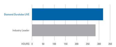
Accelerated wear test conditions: 1200 RPMs, 100 lbs. of tension, 5.2 chain horsepower and 23T x 23T sprockets.
