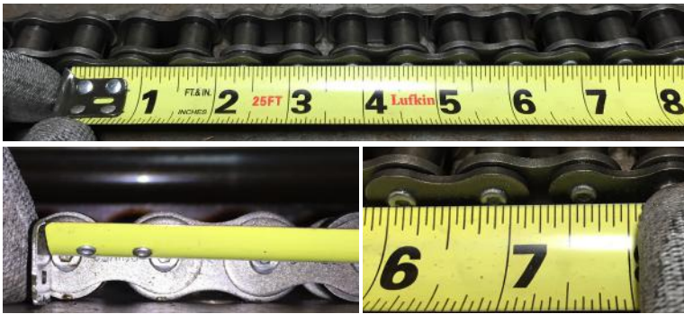
Figure 2: Measuring 10 Pitches of 60-1 Chain with a Tape Measure
