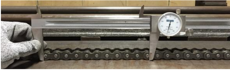
Figure 1: Measuring 10 Pitch Section with a Caliper
