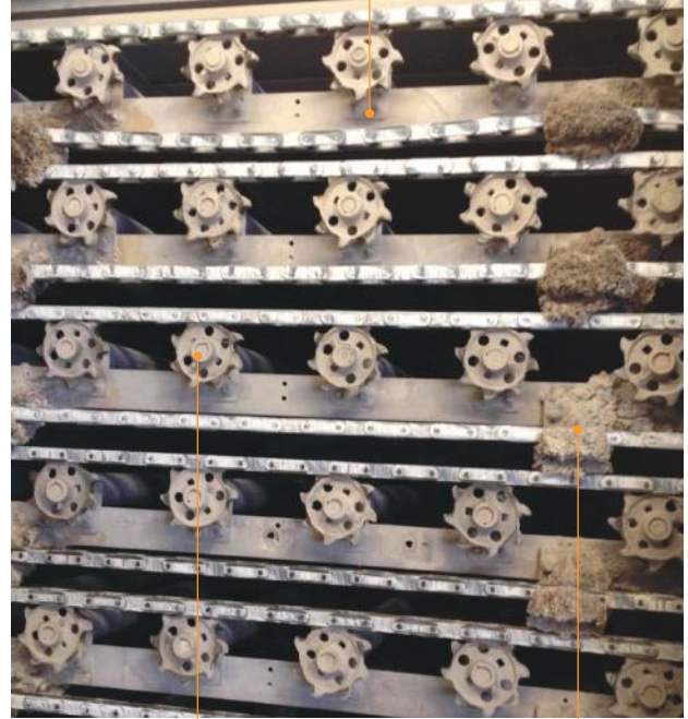
Hook-tooth sprockets rotate the rollers in the oven
